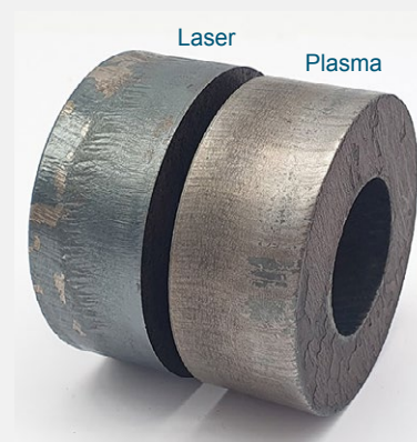
Comparison of cut surfaces 1 inch mild steel
