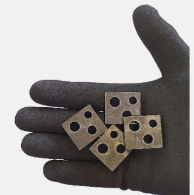
Plasma cutting of small holes
