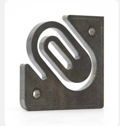
Plasma cutting of fine contours
